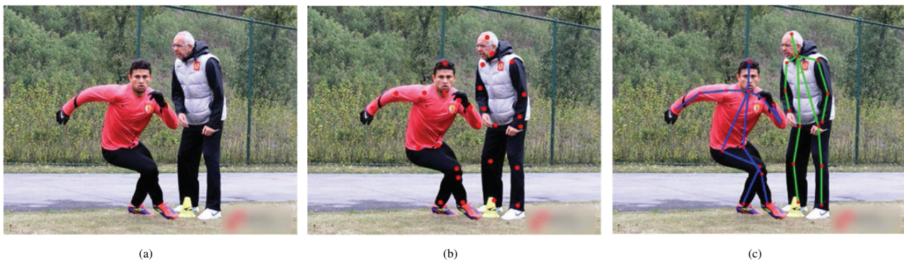
Fig. 11 An illustration of bottom-up pipeline. (a) Input image, (b) keypoints of all the person, and (c) all detected keypoints are connected to form human instance.
