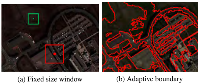
Fig. 2 Spatial region selection by (a) fixed-square window and (b) adaptive boundary adjustment-based segmentation.
