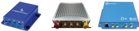
Fig. 3 Experiment devices from left to right: Cohda Wireless Mk5, LTE-V device from DTT, and CWAVE-Original from Nebula Link to the upper computer.
