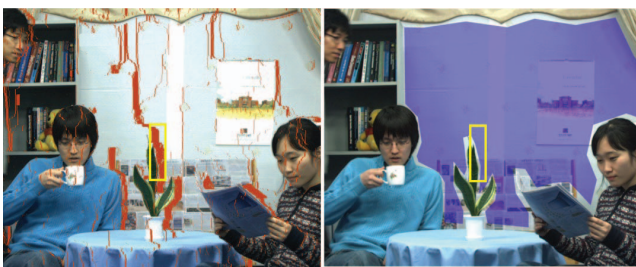
Fig. 8 Depth aware candidate search for patch-based inpainting, with which reference patches of the disoccluded areas (see the yellow rectangle) are preferred from the background (see the purple area in the right sub-figure).
