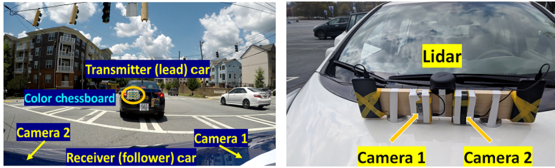
Fig. 2 Experiment setup involving the lead (transmitter from Ref. [6]) and follower (receiver) vehicle. The driving roadways are highway (speeds 80–105 km/h), local road (speeds 40–72 km/h), and parking lot (speeds 8–40 km/h).
