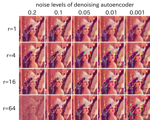
Fig. 12. Reconstructing the color image of “Lena” with 99% pixels missing for the various values of r and noise level.
