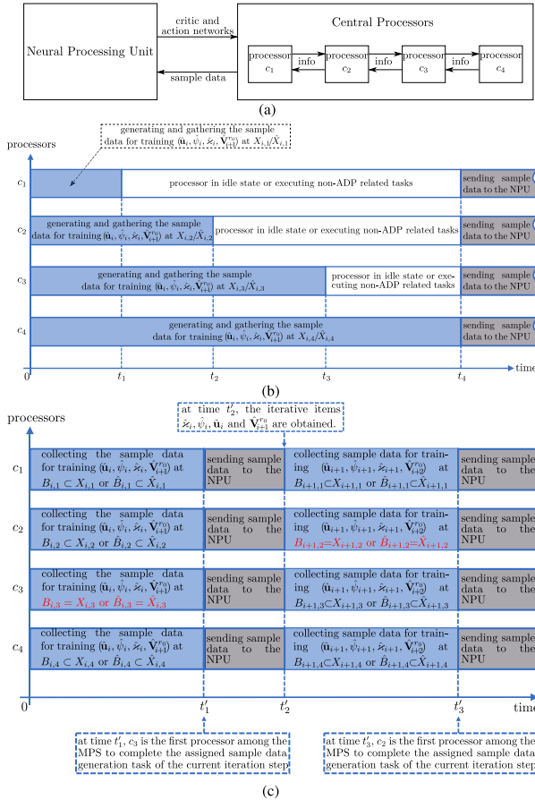
Fig. 5. Comparison between the concurrent ETIADP and HEIADP algorithms. (a) Simplified architecture of the MPS. (b) Task scheduling for processors with the concurrent ETIADP algorithm implemented in the MPS. (c) Task scheduling for processors with the concurrent HEIADP algorithm implemented in the MPS (for illustration purpose only).
