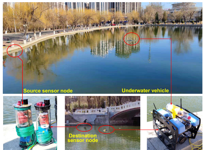
Fig. 8. Experiment deployment, where an underwater vehicle, a source sensor node, and a destination sensor node is included.
