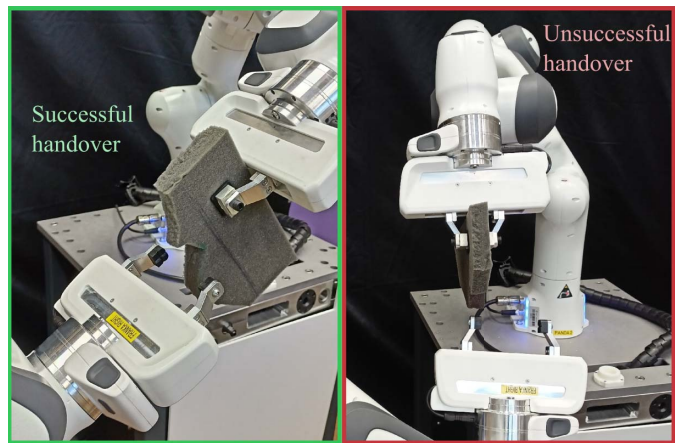
Fig. 11. Example of a successful and an unsuccessful attempt of a robot-to-robot object handover, implemented using RIMEDNet with convolutional layers from AlexNet. The images were taken before the final approach of the receiver robot to grasp the object. The left example shows an accurate prediction of the goal pose, while the grasp attempt on the right image would fail after the approach of the receiver.
