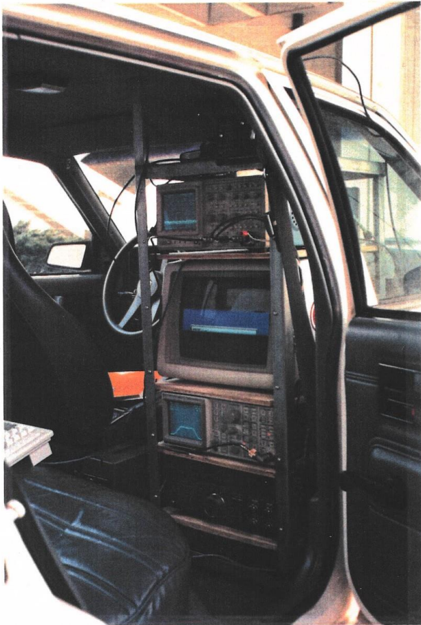
Fig. 4. Full size van converted into a mobile platform to perform impulsive noise measurements in the early 1990s [5]. Power equipment was located in the back area of the van.
