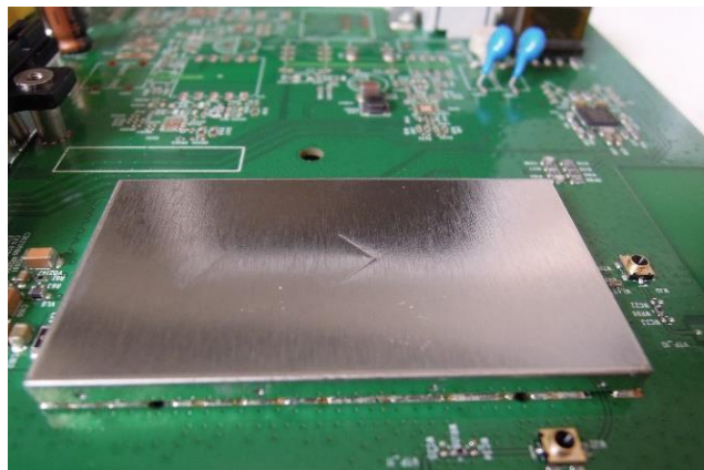
Fig. 1. Board level shield on a Wi-Fi router.
