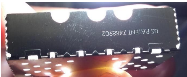
Fig. 12. Sample 1 with back illumination showing gaps where lid joins and corners of the sides
