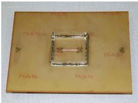
a) with shield lid removed showing stripline
