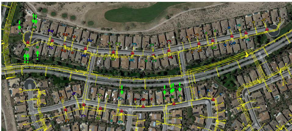
(c) Distance along the street (DAS) metric guides the algorithm on how the distribution line extends from one section to another, following the street. The corrected results are marked with green arrows.
