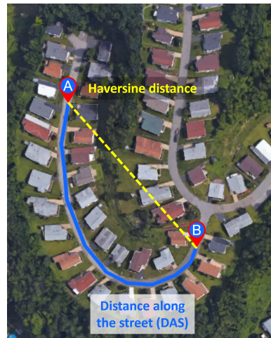
Fig. 4. Comparison between the Haversine distance (dashed yellow line) and distance along the street (solid blue line).
