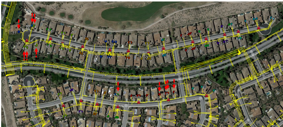
(b) Regular spectral clustering with voltage magnitude only does not work well in scenarios with high PV penetration due to voltage magnitude similarity. Erroneous results are marked with red arrows.
