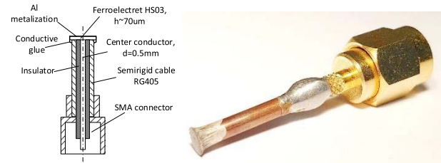
Fig. 1. Microphone construction (left) and the assembled device (right).
