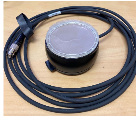
Fig. 5. Coupling pad with imbedded rim, mated to the transducer. Note that the air bubbles seen between the gel pad and transducer face would be removed before use.
