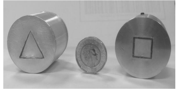
Fig. 13. SG fractal (left) and conventional composite (right) ultrasonic transducer.
