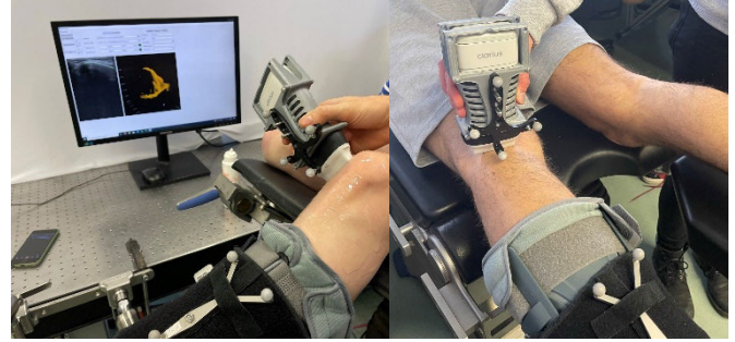
Fig. 2. Experimental setup. The subject's leg is fixated by an adjustable boot. The subject's leg and the wireless probe are tracked by an optical tracking system. Our custom user interface shows the current US image and the recorded 3-D point cloud. Left: anterior scan with the subject in a sitting position and 90° knee flexion. Right: posterior scan with the subject in a prone position and the knee in extension.
