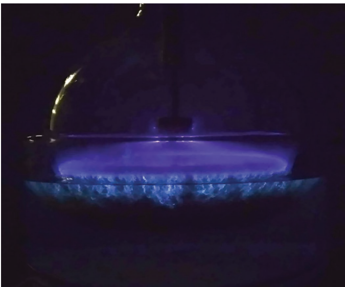
Figure 2. Surface and internal discharges in a highly aged natural ester fluid under low energy discharge. Image courtesy of: Dr. U. Mohan Rao, University of Quebec at Chicoutimi, Canada.
