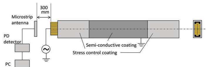
**Figure 2.** Test bar sample, which simulates a real stator coil in a turbine generator.
