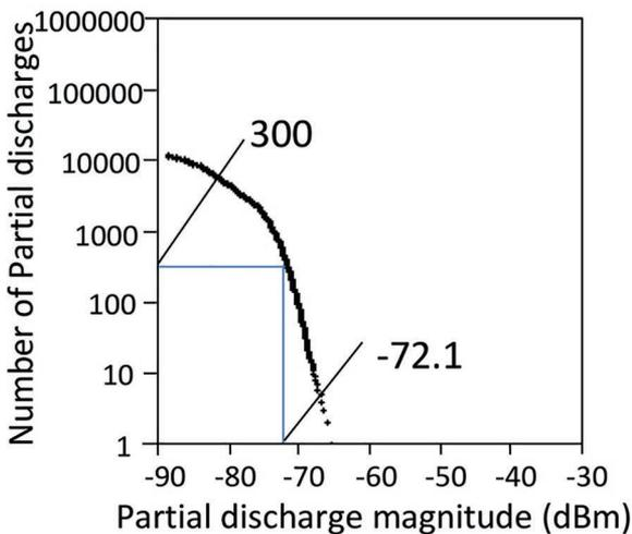
**Figure 4.** Examples of PD measurement results; (a) Phase-resolved intensity, (b) Intensity distribution of the PDs, recorded for 5 s.
