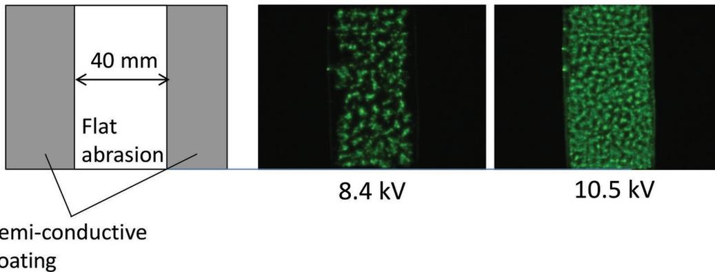
**Figure 6.** Photoluminescence images observed when ac 8.4 or 10.5 kV was applied to the planar abraded hollow shown in the leftmost column.
