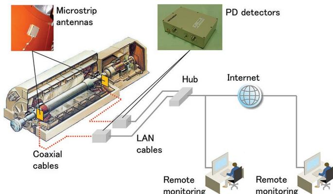
**Figure 1.** Schematic diagram of a monitoring system to confirm the status of electrical insulation in turbine generators.
