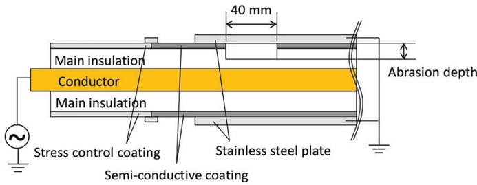
**Figure 3.** Cross-section of the test bar sample used for examining the effects of a planar abrasion of insulation.
