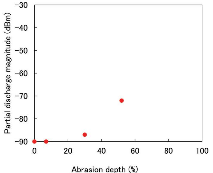
**Figure 5.** Relation between the PD intensity and the depth of the planar abrasion.
