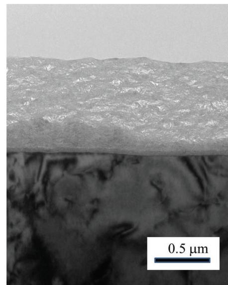
**Figure 4.** Bright field transmission electron microscopy image of the cross-section of the interface between the clay coat and the stainless steel.
