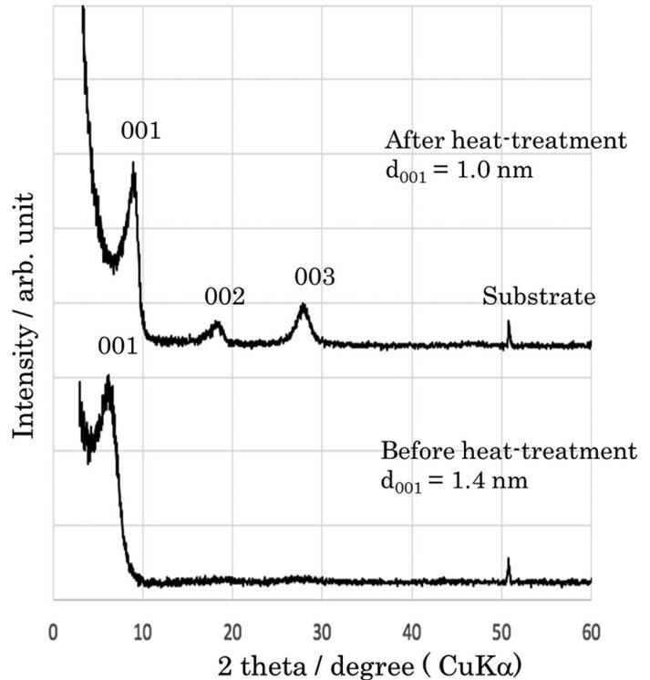
**Figure 3.** X-ray diffraction patterns of stainless steel plates coated with the developed aqueous clay paste, before and after heat treatment at 600°C.
