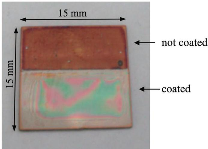
**Figure 2.** Stainless steel plate after the heat treatment at 600°C in air; the lower half was coated with the developed clay coating.
