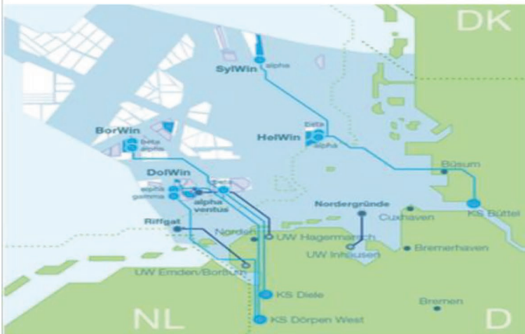
Figure 2. Major high voltage DC (HVDC) cross-linked polyethylene cables already commissioned or under completion in the German North Sea. Courtesy of Prysmian.
