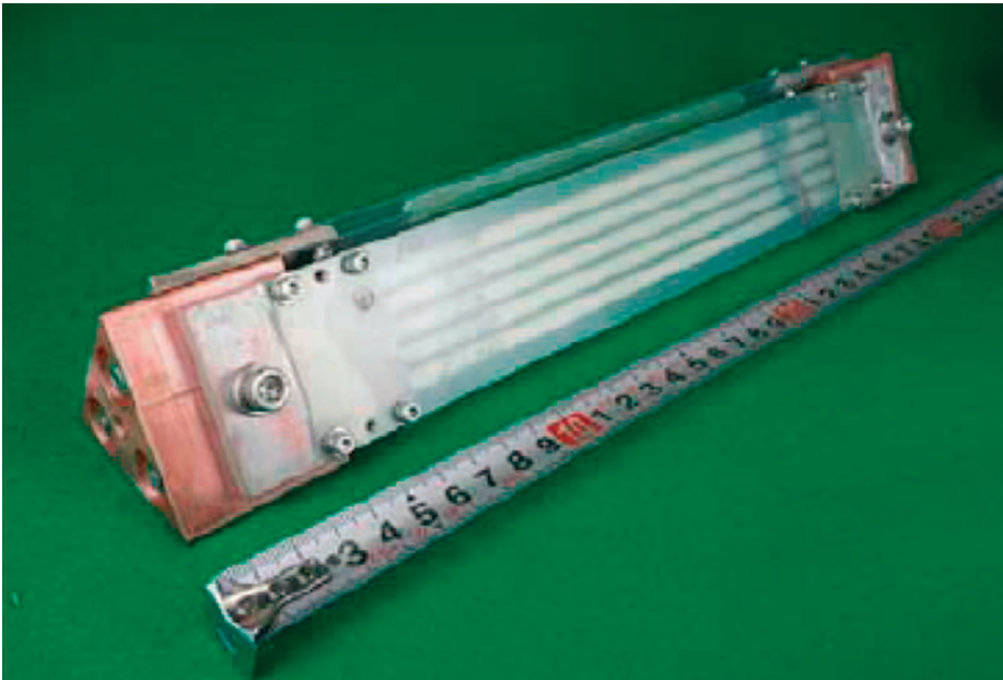
Figure 3. A 1.0-kA HTSC current lead.
