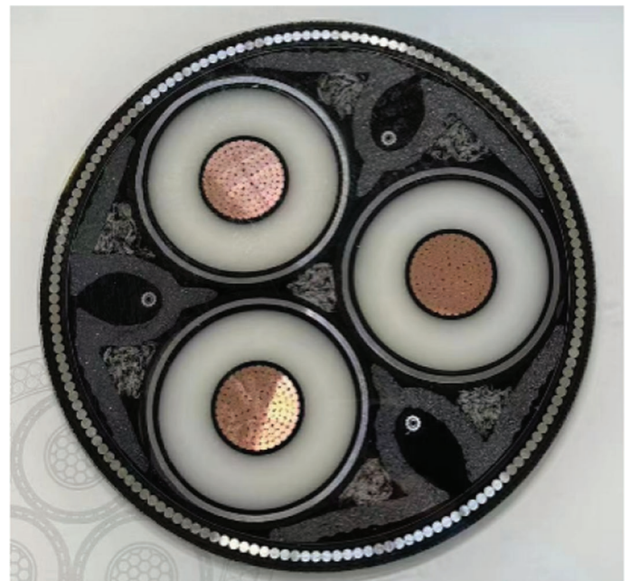
Figure 2. Sectional phase diagram of the 500-kV three-core AC submarine cable.
