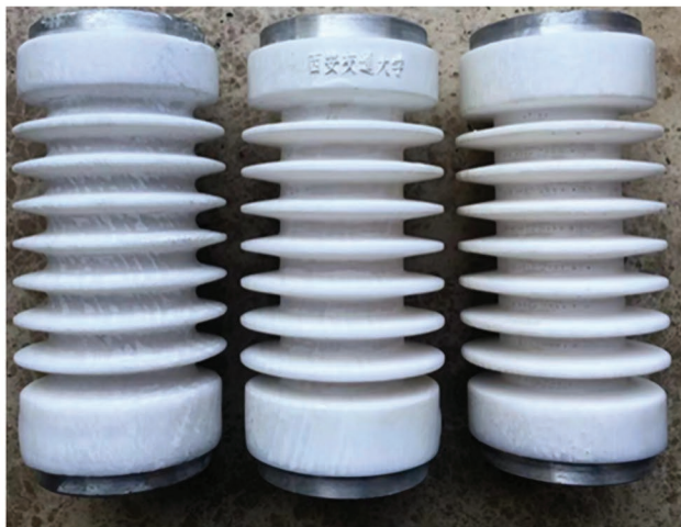
(b) 10kV DGI insulators
