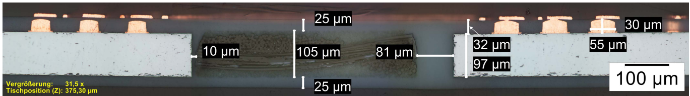
Fig. 5. Cross section of dies embedded in an organic laminate matrix with Cu RDL on top fabricated by semiadditive processing and adaptive direct imaging (DI).
