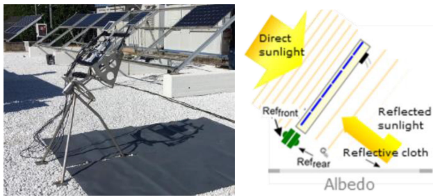
Fig. 4. Outdoor setup using different reflective grounds.
