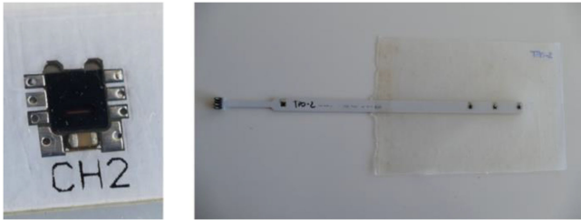
Fig. 1. Miniature sensor (left) and sensor strip in the encapsulant (right).
