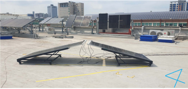
Fig. 8. Experiment with the inclination angle of 30^\circ , with azimuth angles of 240^\circ and 60^\circ .
