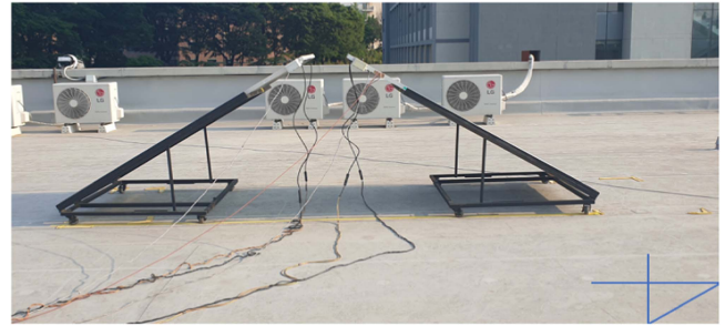
Fig. 7. Experiment with azimuth angles of 90° and 270°, with the inclination angle of 60°.
