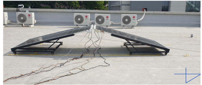
Fig. 6. Experiment with azimuth angles of 90° and 270°, with the inclination angle of 15°.
