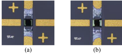
Fig. 7. Microscope images of cells placed on receiving pad I with a solder volume of (a) 16 nl and (b) 29 nl after reflow melting. For all solder volumes the solder flows along the tracks.
