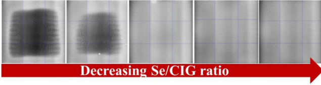
Fig. 6. Optical scanned images for absorber appearance as a function of varying the Se/CIG ratio.
