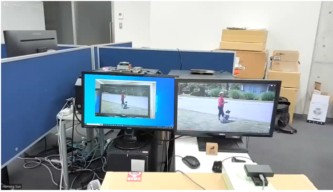
Fig. 7. A demo system for learned image compression. Encoding is performed on an FPGA board KU115, while decoding is performed on an FPGA board VCU118. The links of demo videos are given in the footnote.
