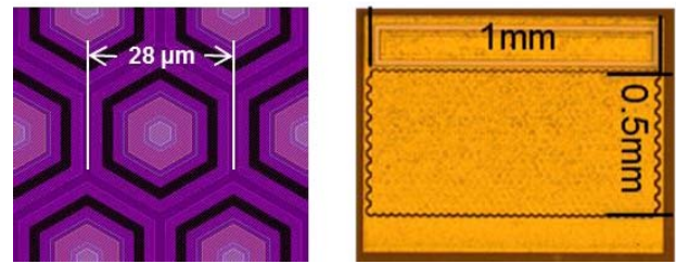
Fig. 2. Top view schematic of the hexagonal layout design; microscopic photograph of a fabricated devices.
