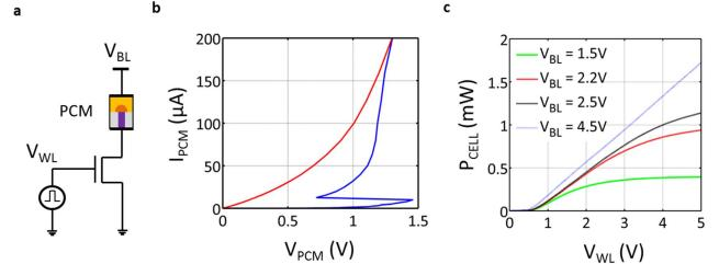
Fig. 1. **a** Schematic of the PCM device used in this work. The subscripts BL and WL refer to the bit line and word line, respectively. **b** Representative  $I$ - $V$  characteristic of a PCM cell employed in this study. **c** Variation of power dissipated in the PCM cell as a function of  $V_{WL}$  and  $V_{BL}$ .
