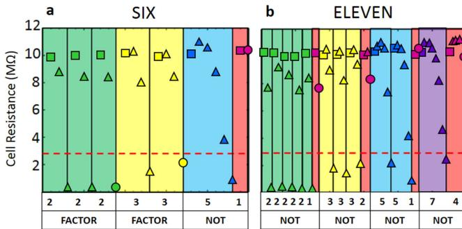
Fig. 4. Finding factors of the numbers 6 and 11, **a** and **b**, respectively, using a single PCM cell. Squares indicate RESET states, triangles intermediate resistance states and circles the end state of a particular factorization test sequence.
