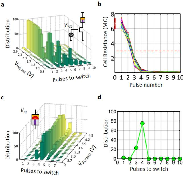
Fig. 2. **a** The effect of  $V_{WL\ EXC}$  on the accumulation properties of PCM cells. **b** The variation of cell resistance versus pulse number for the  $V_{WL\ EXC} = 1.4$  V series (note that data for pulse '0' are the initial reset state resistances). **c** Effect of increasing  $V_{BL\ RESET}$  on the accumulation properties of PCM cells. **d** An extract from c, for  $V_{BL\ RESET} = 2.6$  V.
