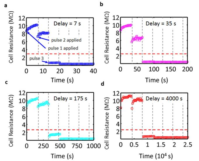
Fig. 3. Accumulation-based computing: a time domain stability study of the intermediate states with a PCM cell. Identical excitation pulses are applied while instructing the control algorithm to wait a specific amount of time (in seconds) between pulses. Increasing time delays of **a** 7 s, **b** 35 s, **c** 175 s and **d** 4000 s are investigated; no substantial difference is observable; the cell switches reliably after 3 pulses.
