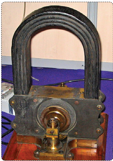
FIGURE 8 The permanent magnet driving dc motor showing a handsome U-shaped magnet.
