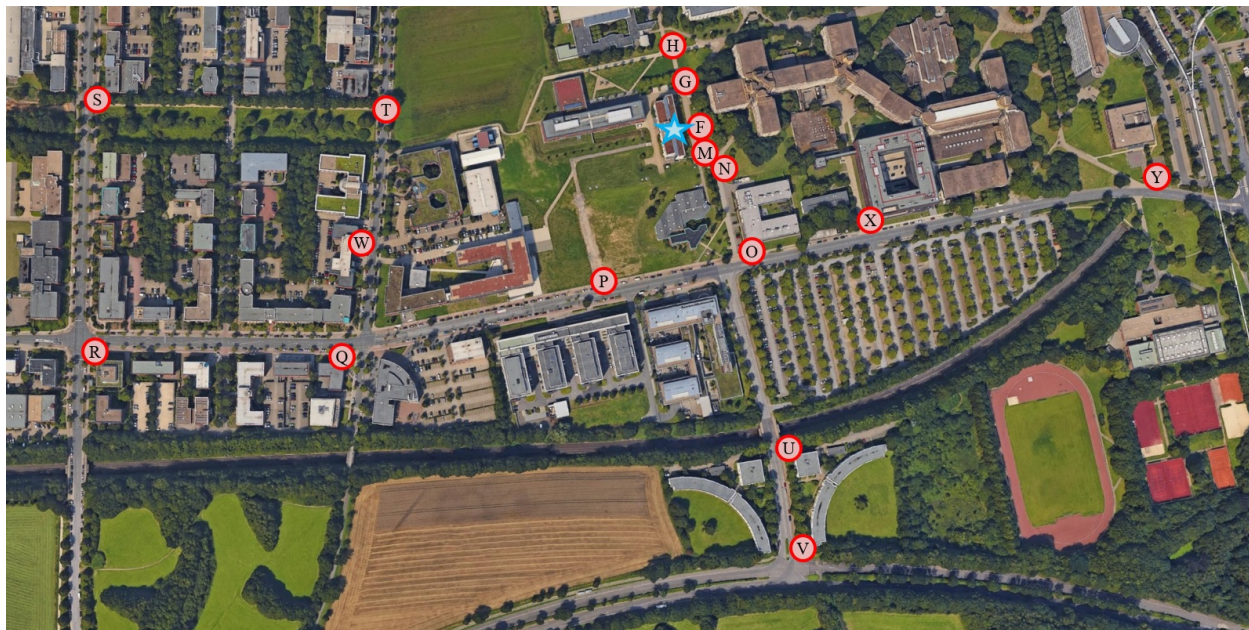
Fig. 2. Receiver locations (RxSites), red circles, in the surroundings of ET Building for Tx-Rx separation above \approx 15 m, common to three installations of the transmitter (TxSites: ‘basement-0’, ‘InHouse’ and ‘Outside’), a blue star.
