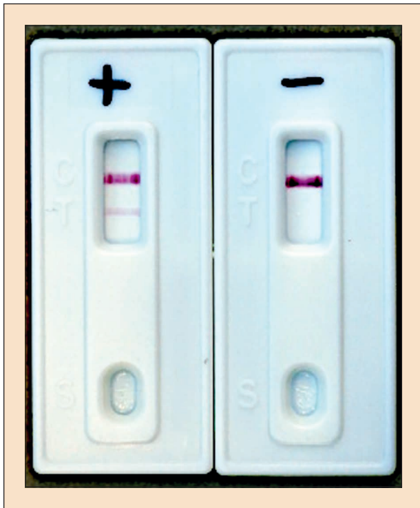
Fig. 4. Human Blood Identification test (ABACard® Hematrace): left strip shows a positive reaction to human blood, while the right strip indicates a negative reaction; the upper, darker purple line is a control band indicating that the test worked properly, and the lower, lighter purple band, visible only on the positive reaction to the left, is the test band that appears if human blood is detected.
