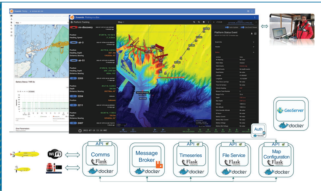
FIGURE 4. An example of how we have reconfigured our microservice system to accommodate the case of piloting from a ship. We have adapted our microservices to connect directly to the hardware in the ship (in this case, the RSS Discovery) using our communication microservice, we wrote integrations for Wi-Fi, to talk to the AUVs when on deck or in the water near the ship, and then USBL (ultrashort baseline, an underwater acoustics system), to track the AUVs underwater and send short commands to them (like emerge or start a mission). The example shown is during the cruise DY152. The integration of GeoServer allows us to show layers locally without needing an Internet connection; in the map on the piloting in a box app, we are showing high-density bathymetric layers provided by the ship instruments.
