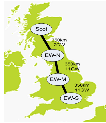
Fig. 4. Schematic topology and the existing capacity of the GB transmission links between the key regions.
