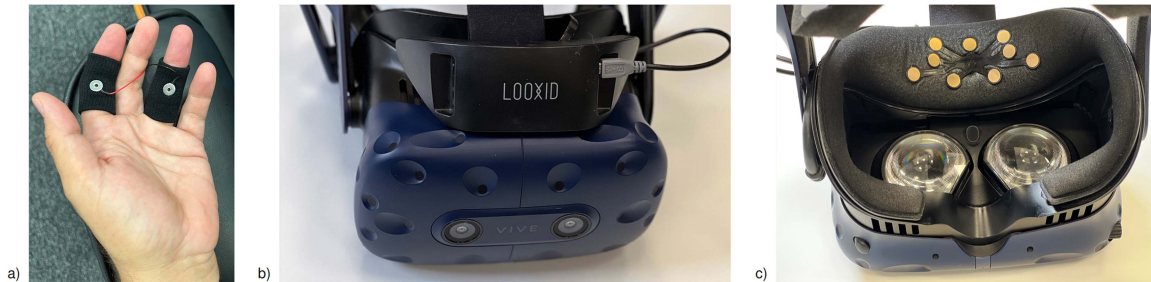
Fig. 4. Biosensors used in the research: a) GSR b) Looxid Link - outside view of the glasses c) Looxid Link - inside view of the glasses.
