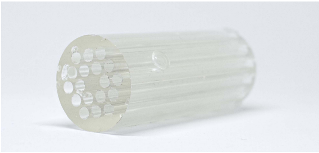
Fig. 3. Photograph of structured preform (PR2b) with two rings of airholes (18 holes in total) and a length of 75 mm.
