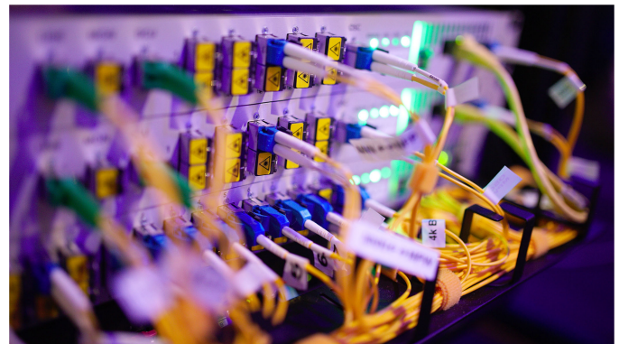
Fig. 9. Close-up of a Czech Light ROADMs at the TIP Summit in London (October 2018).
