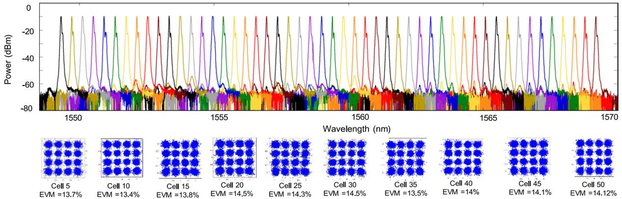
Fig. 8. Spectra of switched optical SSB signals and examples of signal performance at different cells.
