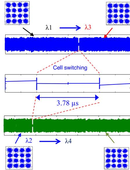
Fig. 7. Cell switching by the wavelength-tunable lasers.
