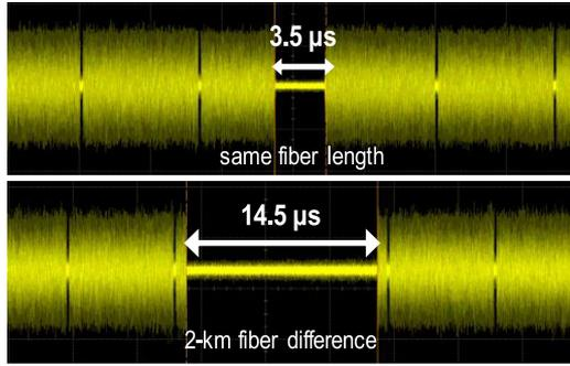
Fig. 12. The interrupted time during radio cell switching.
