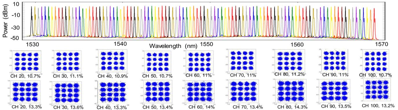
Fig. 11. Spectra of the switched optical SSB signals and examples of the signal performance for systems using 10-km SMF (upper) and 20-km SMF (lower).
