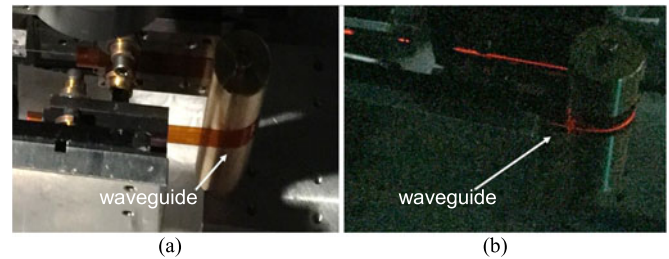
Fig. 4. Images of the bent waveguide sample (a) under room lighting and (b) illuminated with red light.
