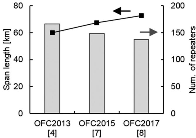
Fig. 7. Expected reduction in repeater numbers in 10,000 km, 8QAM-150G ( $Q \geq 7.0$  dB) system.
