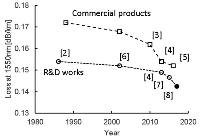
Fig. 1. History of improvement in losses of Ge-free silica core optical fibers measured at 1550 nm wavelength.
