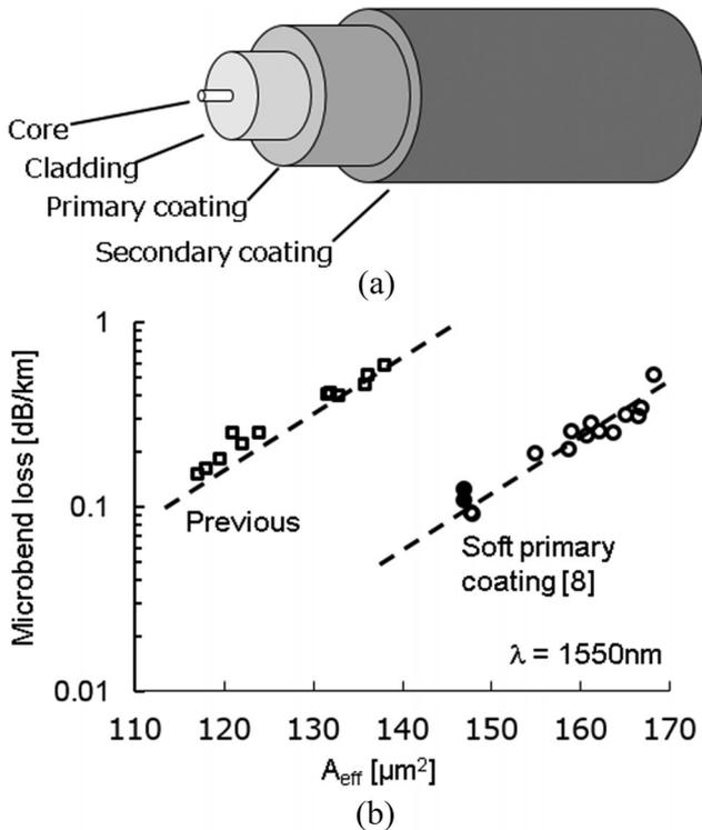
Fig. 5. (a) Schematic diagram of polymer coatings surrounding glass of optical fiber. (b) Correlations between microbending loss measured on wire mesh drum test and effective area, for different coatings.
