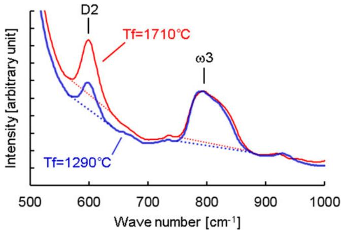
Fig. 3. Raman spectra of two optical fibers with different fictive temperatures. The dotted lines show assumed base lines to define peak areas.
