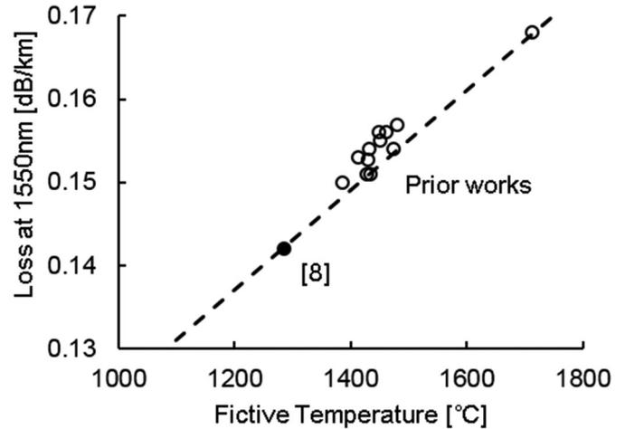
Fig. 4. Correlation between fiber loss and fictive temperature by Raman spectroscopy.
