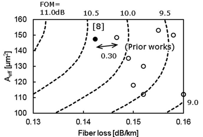
Fig. 6. FOM contour map for an 80 km span system. The solid and open plots show the present and previously reported works, respectively. The dashed lines show contours of FOM value represented as Q-factor assuming QPSK-100G transmission.
