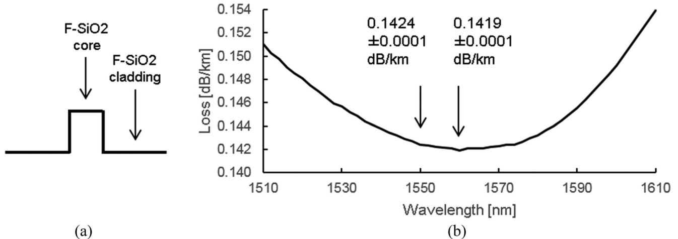
Fig. 2. (a) Schematic index profile of the fabricated fiber. (b) Its transmission loss spectrum by the cutback method. The inset values show the mean and standard error of 10-time cutback measurements.
