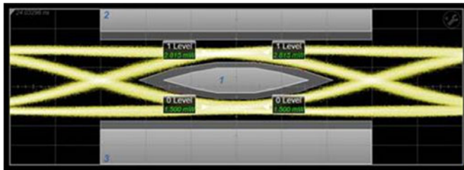
Fig. 5. Typical eye diagram from a 28 Gb/s transceiver demonstrating more than 30% margin the standard defined mask.
