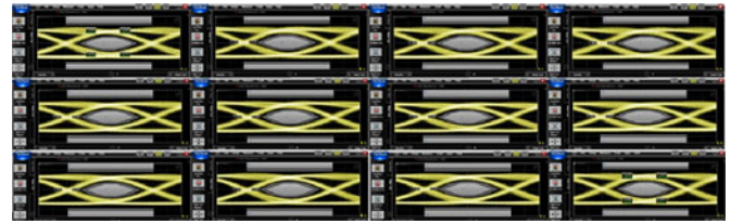
Fig. 7. Optical eye diagrams from a 12 \times 25 Gb/s transceiver demonstrating more than 25% mask margin on every channel with all channels running.
