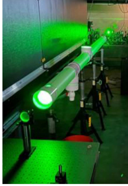
Fig. 8. The double pass through a 3 m underwater channel. The effects of scattering can be seen in the light illuminating the walls of the tube.
