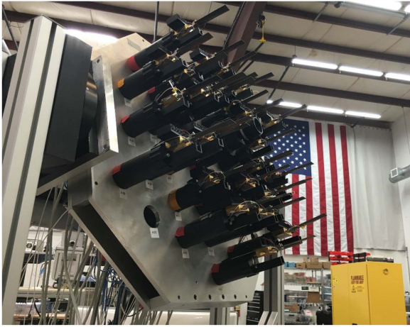
Fig. 1. Two-dimensional antenna array with aperiodic antenna positions for alias-free imaging.
