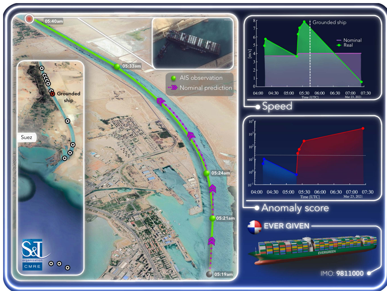
Fig. 1. Overview of the automatic anomaly detection tool applied to the real-world scenario of the Suez Canal blockage [19]. The Ever Given trajectory reported by AIS from 23-03-21 to 29-03-21 is displayed on the left. In the middle panel, the nominal trajectory and the AIS observations are depicted right after the entrance of the canal and before the grounding. On the right panels, the anomaly score is reported as well as the nominal and the real speed of the ship. The alarm is triggered (red dots) when the score is above the threshold (white dotted line), while the nominal condition is declared (blue dots) when the score is below the threshold. Credit: Satellite image © 2021 Maxar Technologies.
