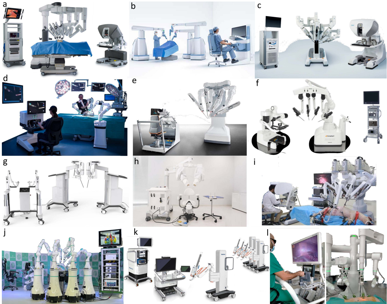
Fig. 1. Most advanced RAMIS systems, featuring only commercially available, and ready-to-launch platforms, already cleared for at least a limited set of surgical indications (presented in the order of time of appearance). (a) da Vinci Xi. (b) Senhance Surgical Robotic System. (c) Revo-i. (d) Versius. (e) Avatera. (f) Hinotori. (g) Dexter. (h) Symani Surgical System. (i) Toumai Endoscopic Robot. (j) Mantra. (k) Hugo RAS System. (l) Bitrack. Table 1 at the end provides details regarding these robots' basic engineering and clinical capabilities. (Image credit: the manufacturers.)
