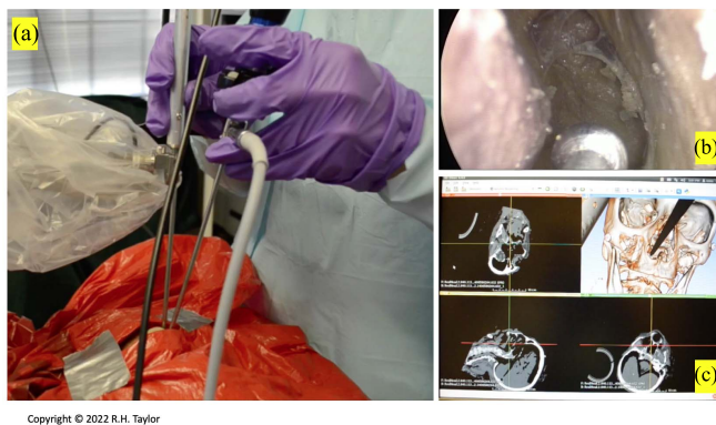
Fig. 10. Hand-over-hand cooperative control with virtual fixtures for sinus surgery. In this experiment, (a) the surgeon manipulates a pointer tool held by the robot while (b) observing the tool through endoscopic video. (c) The system uses a registered model of the tool-to-anatomy relationship to help guide the tool to its desired target while ensuring that it does not collide with delicate structures [57], [58]. (Figure copyright (C) 2022 R. H. Taylor.)
