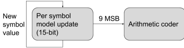
Fig. 26. Probability model is updated and maintained in 15-bit precision, while only the most significant 9 bits are used by the arithmetic coder.
