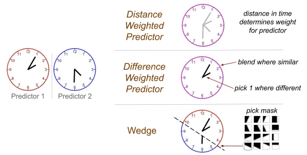
Fig. 13. Illustration of the compound prediction modes. The distance weighted predictor uniformly combines the two reference blocks. The difference weighted predictor combines the pixels when their values are close (e.g., the dial plate and the numbers) and picks one reference when the difference is large (e.g., the clock hands). The wedge predictor uses one of the preset masks to split the block into two sections, each filled with one reference block's pixels. In the above example, it stitches the lower part predictor 1 and the higher upper part of predictor 2 as the compound prediction.
